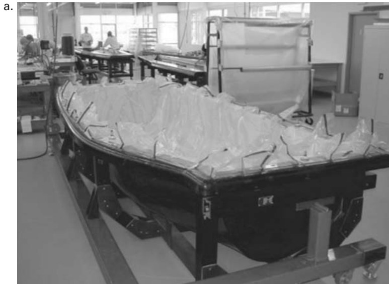
Vacuum bag on fuselage tool
