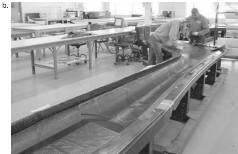
Laying up the carbon material into the tail boom tool.
